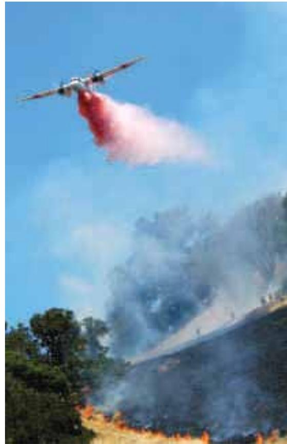
Air tankers offer invaluable assistance to firefighters on the ground, but the fire retardant they carry must be delivered carefully due to its detrimental impacts on waterways. Photograph by P. Armstrong.
